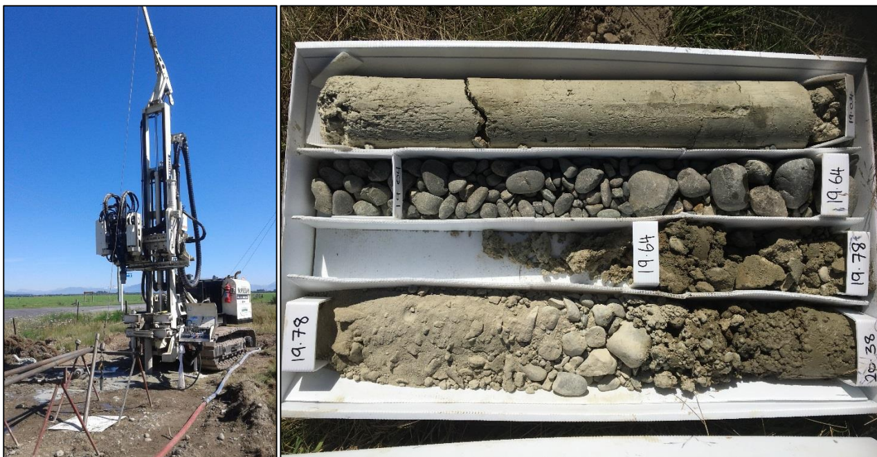
Figure 14: Pilot Trial dedicated monitoring bore drilling programme: Sonic drill rig and boxed core (GWD-1, March 2016).
